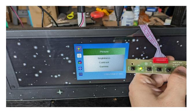
Hit [MENU] again to select the brightness adjustment, use the [LEFT] or [RIGHT] buttons to adjust the brightness up or down.
